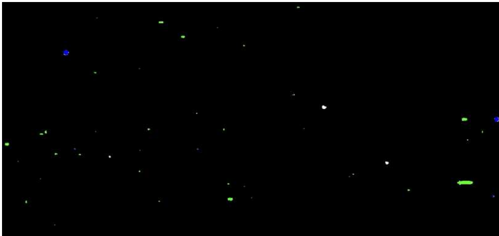
Figure 7.13 Example of shape associations: zoom on BG11 thin-section after binary conversion. Green: ellipses-associated shapes, blue: circles-associated shapes, white: unselected square-associated shapes. Below: rose diagram with ellipse orientations. Note that thin section is oriented normal to the bedding.
