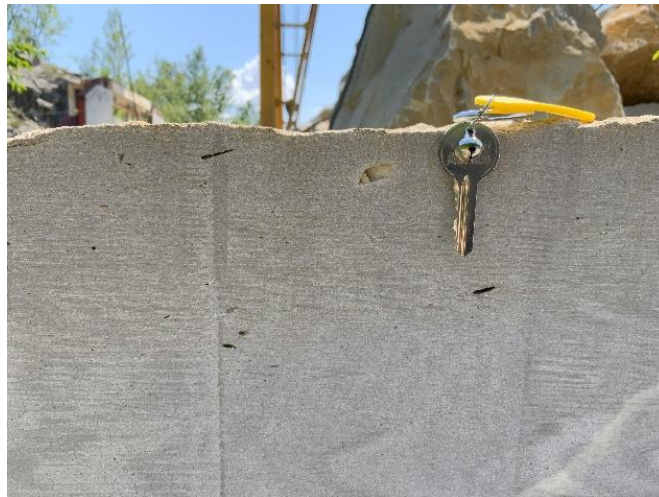
Fig. 4.4 "Pietra Piasentina" calcarenite of Megabed n.3 (Mount Ioanaz Megabed) with clay chips holes. The lines are saw marks.
